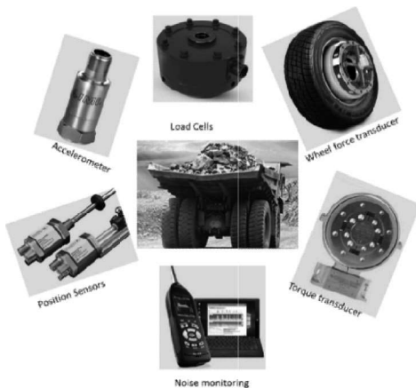
Figure 2 Sensors installed in machines for maintenance information needs
